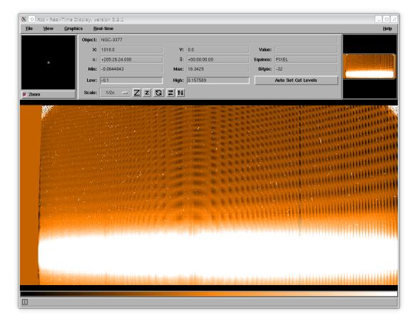
Therefore, the option skymedian is used instead to process LSS data, as shown below . This sky subtraction uses the median of the signal of all pixels in a wavelength bin of the rectified frame as sky signal for that wavelength bin.
