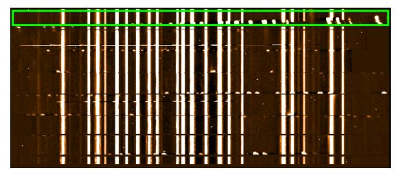
Reducing the peak detection parameter from 300 to 250 allows the pipeline to correctly trace the topmost slitlet:
