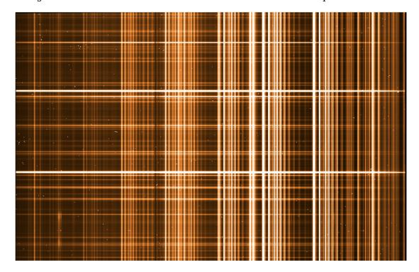
The screen shot above shows the rectified, wavelength calibrated pipeline product for the raw file FORS2.2009-04-28T08:36:27.441 (GRIS\_300I+OG590 observation of V4334 Sgr). The screen shot below shows the frame after the sky subtraction. One can clearly see that too much skylight has been subtracted in the lower part (dark sky lines) and too little in the upper part (bright sky lines). Please note that the dynamic range of the image above is 10 times larger than that of the image below.
