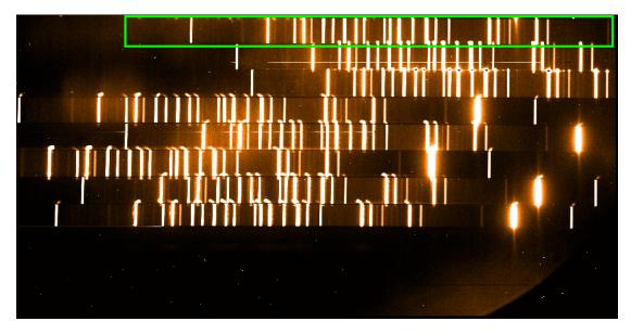
The wavelength calibrated arc lamp frame shows that the topmost slitlet has not been properly detected - it includes lines from the slitlet below:
