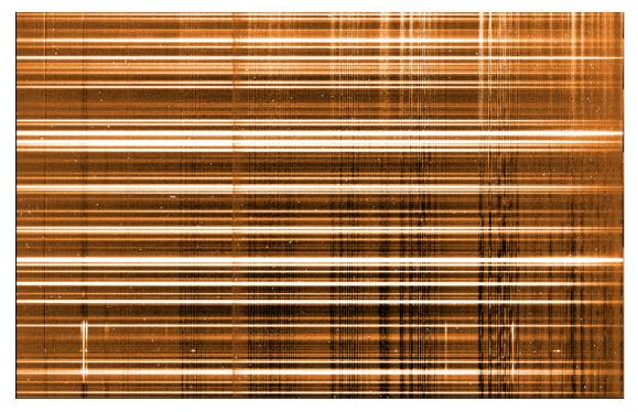
Below we show two spectra extracted from the sky subtracted frame above, from the upper part (too little sky subtracted, sky lines in emission) and from the lower part (too much sky subtracted, sky lines in absorption). While the effect is obvious for these faint spectra it will be more subtle for bright targets.
