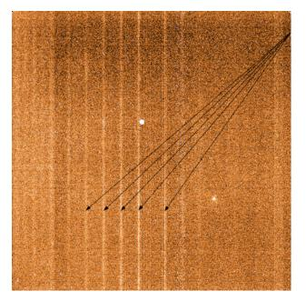
Although the saturation level of the detector is 45000 ADUs, SINFONI observations must keep below about 1/6 of that to avoid detector persistence. Detector persistence would affect the subsequent observations of faint sources, and can take days to disappear, therefore this must be avoided. The current detector persistence
